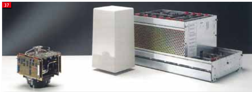
▲ Figure 37. XTV 8 camera (left) compared with vidicon camera and control unit (right).
